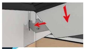
Lift transom rafter and offer the bracket up to the slot in the ridge at an angle. Insert the bracket and then rotate the rafter into position at the ringbeam.
