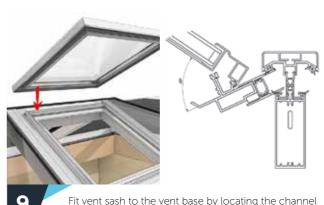
9 Fit vent sash to the vent base by locating the channel in the sash profile into the 2 pivot profiles on either end of the vent base as shown. The sash should be offered at approximately 60° to engage correctly, then rotated down to lock in.
