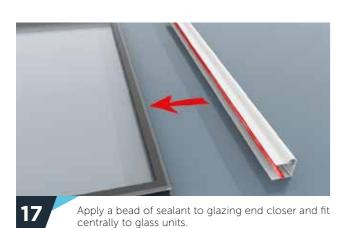
Note: Always use the correct polymer sealant for self cleaning glass.
