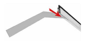
Insert tie bar bracket into the side of one of the central rafters.
