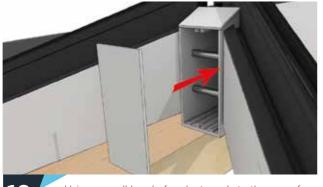
Using a small bead of sealant, apply to the rear of the ridge end closer plate and secure to the cut end of the ridge as shown.
