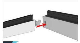
Loosen retention screws in hips and insert the connection brackets into the wider machined slots in the side of the ridge. Return to step 8, fitting the framework into the ringbeam, pushing down the hips to tighten the joints. Tighten retention screws.
