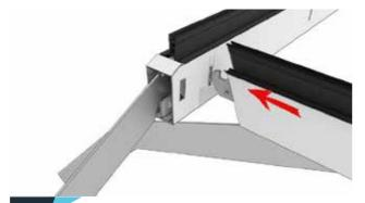
2 Loosen retaining screw from transom connection bracket so that it can move freely and insert transom bracket into slot in the ridge.
