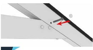
Using a 6mm bit, drill a hole through the rafter and tie bar brackets.
