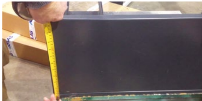
3 Mark out the cornice 70mm and 210mm from the bottom.
