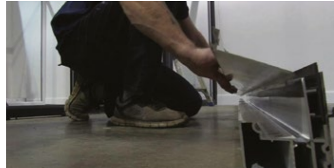
2 Remove the ringbeam flaps from the ringbeam.
