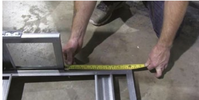
1 Centralise the vertical ladder frame onto the horizontal bottom frame and fix together with the screws provided.
